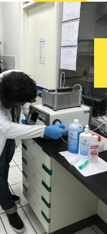
A collaboration was established from the Department of Metrology in Chemistry, to sample and determine the ethanol content in commercial liquid alcohol samples by measuring its density and refractive index. These products must contain at least 60% alcohol to be used as disinfection means.
