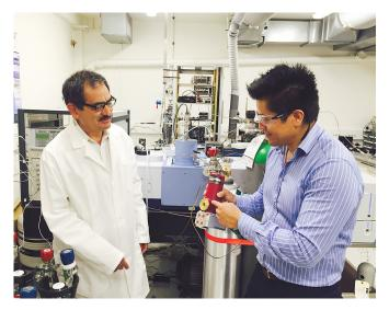
Mr M. de J. Avila (CENAM) with Dr E. Flores (BIPM) in the BIPM gas metrology laboratory, setting up the FTIR system for the comparison of  $CO_2$  gas standards
