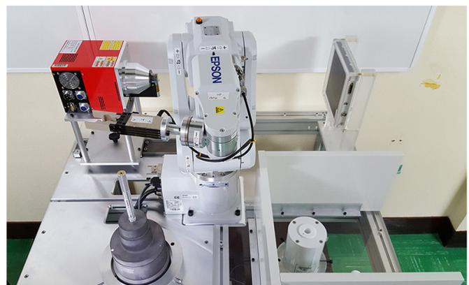
The robotic arm for manipulation of radioactive sources
