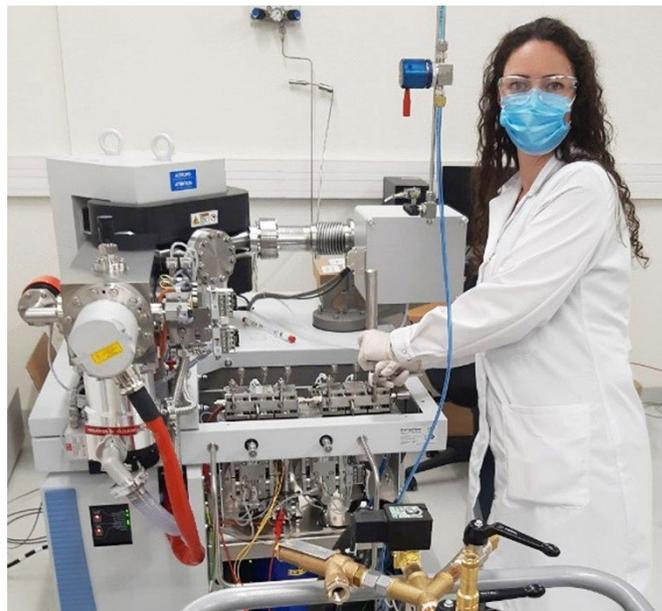
Newly established isotope ratio mass spectrometer facility supporting comparison of CO<sub>2</sub> and CO<sub>2</sub> in air isotope ratio standards, CCQM-P204 and future planned on-demand comparisons BIPM.QM-K3 and BIPM.QM-K4
