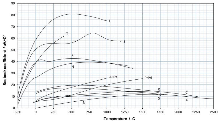
**Figure 3.** The Seebeck coefficient for common thermocouple types.
