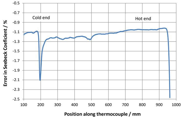
**Figure 14:** The Seebeck coefficient of a Type S thermocouple adversely affected by rhodium migration. Note the large downward spike at 200 mm where rhodium has contaminated the platinum thermoelement.
