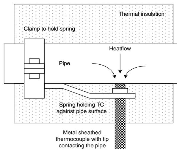
Figure 8: A poor thermocouple installation susceptible to poor thermal connection with the pipe and gradients across the measuring junction.
