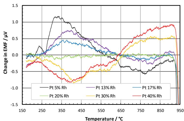
**Figure 4:** Changes in emf ( $t_m = 100^\circ\text{C}$ ,  $t_r = 25^\circ\text{C}$ ) in platinum-rhodium alloys as a function of temperature and alloy composition after 100 hours of exposure at the indicated temperature (Webster 2020).
