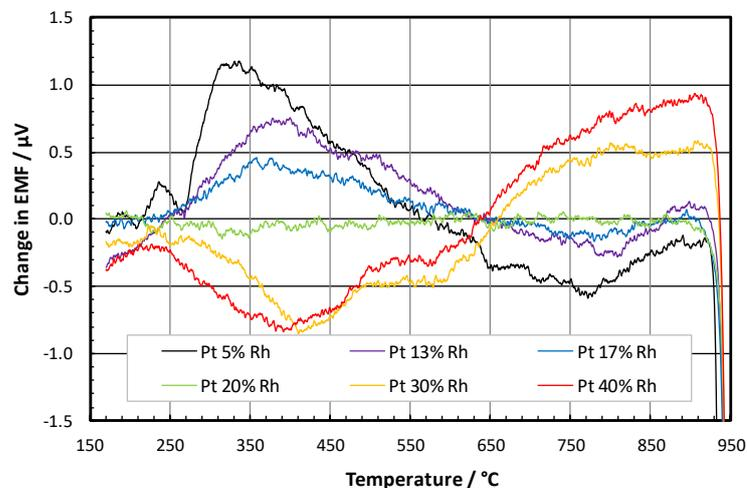
**Figure 4:** Changes in emf ( $t_m = 100^\circ\text{C}$ ,  $t_r = 25^\circ\text{C}$ ) in platinum-rhodium alloys as a function of temperature and alloy composition after 100 hours of exposure at the indicated temperature (Webster 2020).
