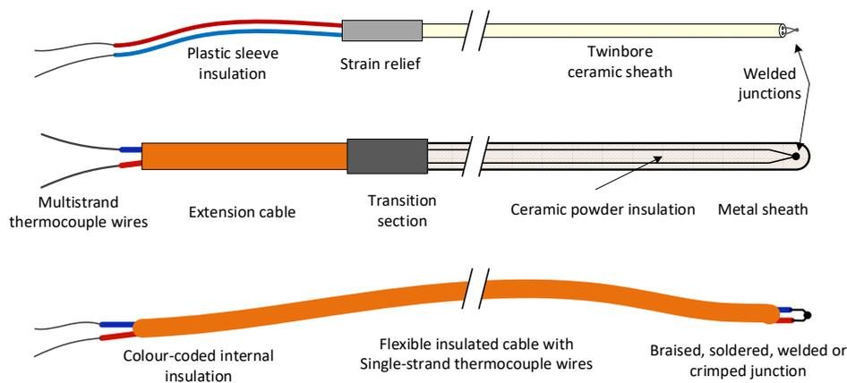
**Figure 5.** Examples of different thermocouple assemblies. Upper: a laboratory standard thermocouple using a hard-fired twin-bore ceramic sheath; middle: a mineral insulated metal sheathed (MIMS) assembly with extension cable; lower: a fully flexible plastic-insulated assembly.
