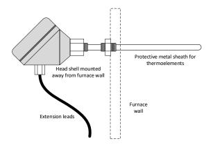
Figure 7: Typical industrial thermocouple installation.
