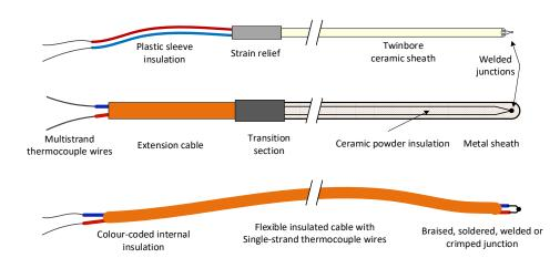
**Figure 5.** Examples of different thermocouple assemblies. Upper: a laboratory standard thermocouple using a hard-fired twin-bore ceramic sheath; middle: a mineral insulated metal sheathed (MIMS) assembly with extension cable; lower: a fully flexible plastic-insulated assembly.
