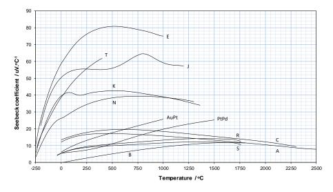
Figure 3. The Seebeck coefficient for common thermocouple types.
