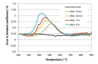
Figure 12: Measured change in Seebeck coefficient in a Type K sample due to ordering, for different operating temperatures and exposure times.
