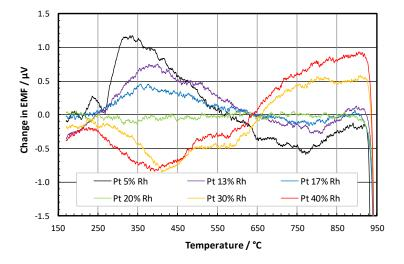
**Figure 4:** Changes in emf ( $t_m = 100 \text{ °C}$ ,  $t_r = 25 \text{ °C}$ ) in platinum-rhodium alloys as a function of temperature and alloy composition after 100 hours of exposure at the indicated temperature (Webster 2020).
