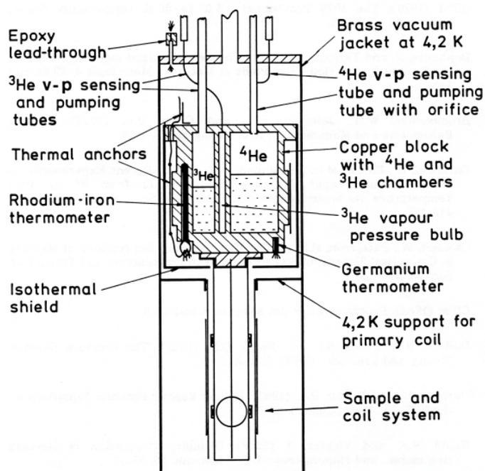
**Figure 3.** A schematic diagram of the cryostat used by Rusby and Swenson [1980] for CMN magnetic thermometry and for  $^3\text{He}$ ,  $^4\text{He I}$  and  $^4\text{He II}$  vapour-pressure measurements. © Bureau International des Poids et Mesures. Reproduced by permission of IOP Publishing. All rights reserved.
