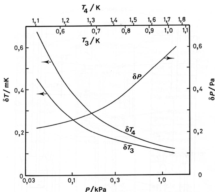
**Figure 1.** Examples of uncertainties in pressure measurements using a capacitance diaphragm pressure gauge below 1.3 kPa, and the equivalent uncertainties  $\delta T_3$  and  $\delta T_4$  in temperatures  $T_3$  and  $T_4$  for  $^3\text{He}$  and  $^4\text{He}$  vapour-pressure measurements, respectively [Rusby and Swenson 1980]. © Bureau International des Poids et Mesures. Reproduced by permission of IOP Publishing. All rights reserved.
