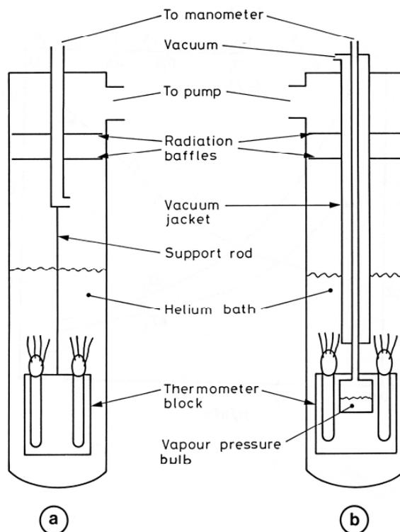
**Figure 2.** Schematic illustrations of systems for realizing  $^4\text{He}$  vapour pressures: using a bath of liquid (a), suitable for  $^4\text{He II}$ , and a bulb (b) for  $^4\text{He I}$ , unsuitable for  $^4\text{He II}$ . Thermal shields around the helium bath are not shown.
