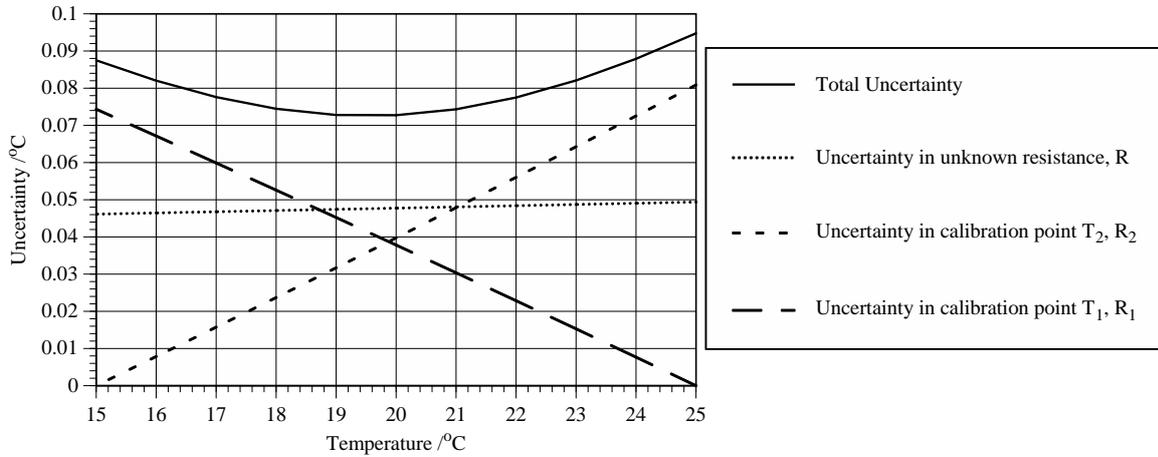
**Figure 5.** The propagation of uncertainty ( $k = 1$ ) for a thermistor calibrated at two points. The numerical data is from Table 2, and the propagation equations for the three contributions are from Equation (17).
