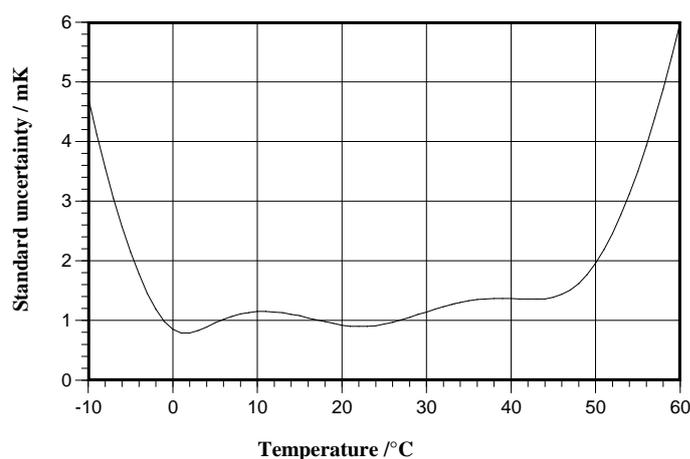
**Figure 6.** The total standard uncertainty ( $k = 1$ ) propagated from the calibration measurements of the thermistor using Equation (11), and the data tabulated in Table 3.
