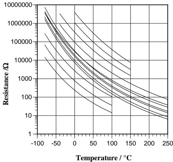
**Figure 1.** The resistance-temperature characteristics for a range of thermistors showing the typical resistance and temperature ranges.
