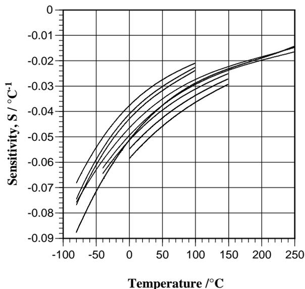
**Figure 3.** The sensitivities, Equation (4), as a function of temperature for the thermistors of Figure 1.
