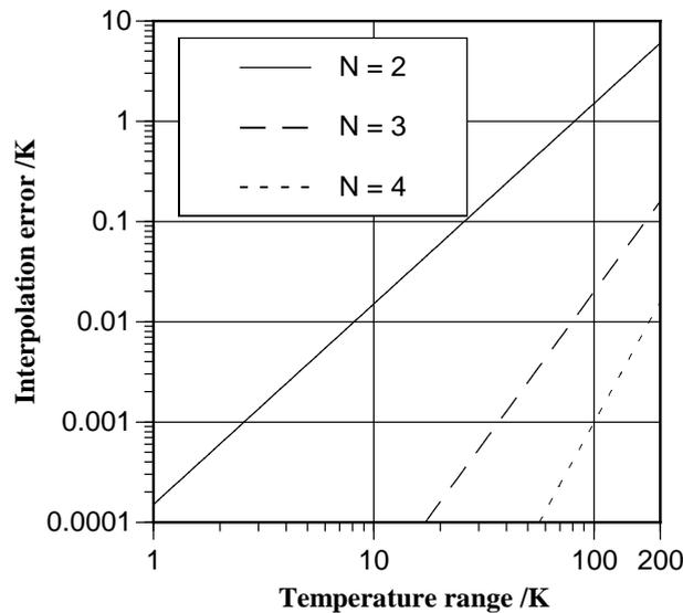
**Figure 4.** Summary of interpolation errors, expressed as standard uncertainty, versus the number of terms used in Equation (9). The lines are indicative only and are based on a thermistor with a  $\beta$  value of 3800 K. The error will tend to be greater for temperatures below  $0\text{ }^{\circ}\text{C}$ , for thermistors with a high  $\beta$  value, and may vary by a factor of 2 or more for different thermistors.
