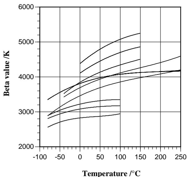
**Figure 2.** The  $\beta$  values for the thermistors of Figure 1. Some of the thermistors have the same  $\beta$  value.
