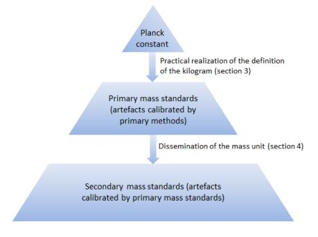
Figure 1. Illustration of the traceability chain from the definition of the kilogram. The unit of the Planck constant being  $kg m^2 s^{-1}$ , the units second and metre are needed to derive a primary mass standard from the Planck constant.
