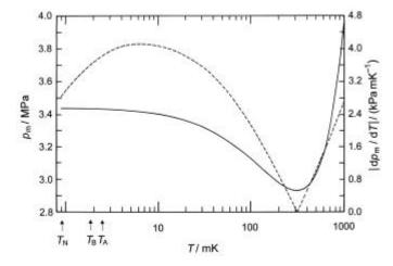
Figure : The  $^3$ He melting pressure p (full line) and the absolute value of the derivative dp/dT (dashed line) vs. temperature.  $T_{\rm N}$ ,  $T_{\rm B}$  and  $T_{\rm A}$  indicate the temperatures of three phase transitions in solid or liquid  $^3$ He.
