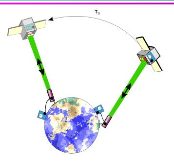
**Common View** No noise added from the onboard oscillator
