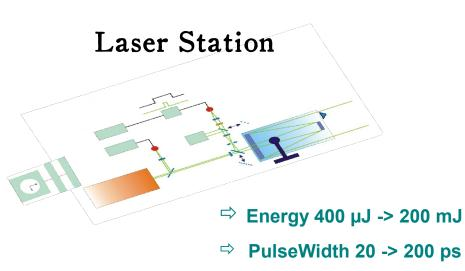
Comparison between ground to space time transfers coming from the whole laser station network permits to realize ground to ground time transfer
