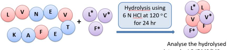
Spike isotope-labelled Phe, Val and Leu (F\*, V\* and L\*) as internal standards Analyse the hydrolysed mixture by LC-IDMS/MS using Phe, Val and Leu (F, V and L) CRMs as calibration standards
