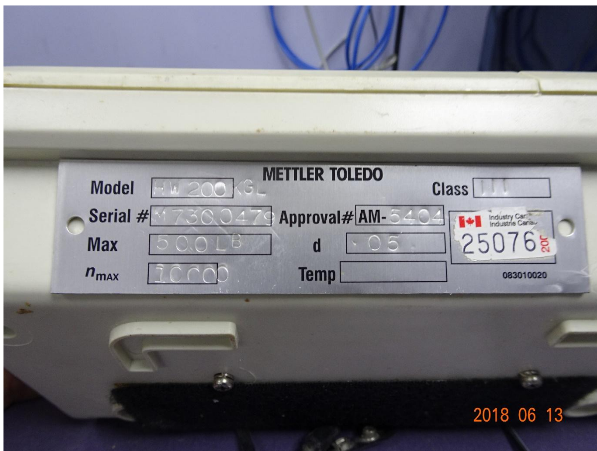
Figure 2. A weighing instrument manufactured in Australia with a Measurement Canada approval mark as an apparent forged information plate.
