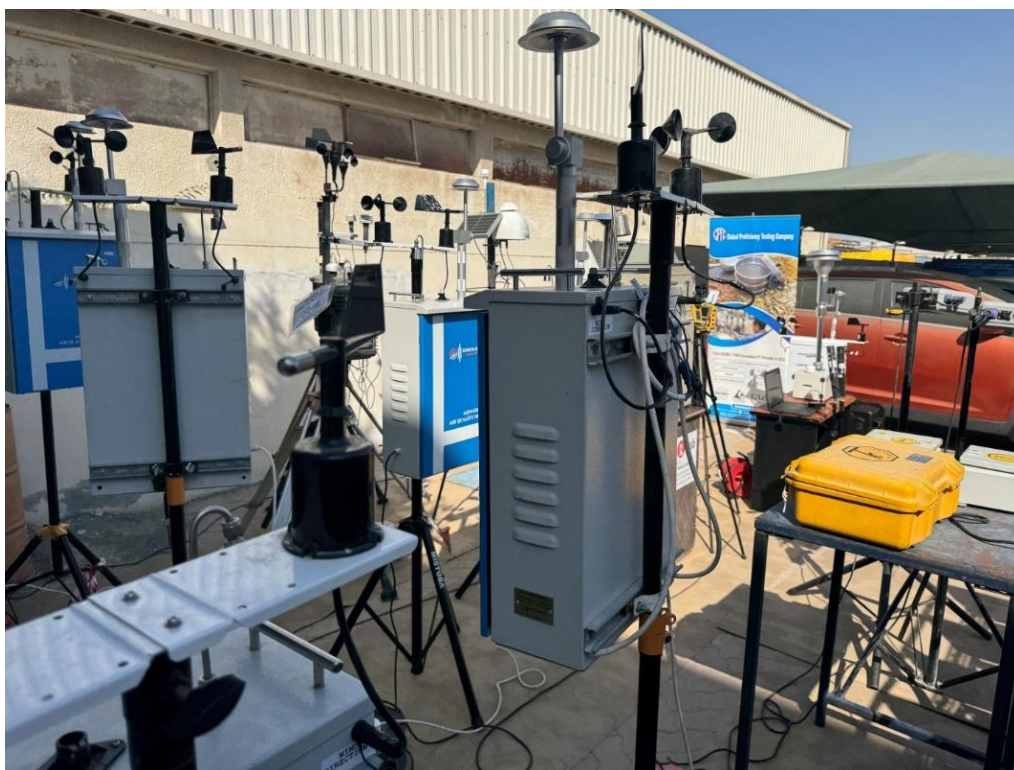
Figure 2. Air monitoring stations are used for proficiency testing (PT) of outdoor ambient air quality monitoring, conducted in industrial areas.
