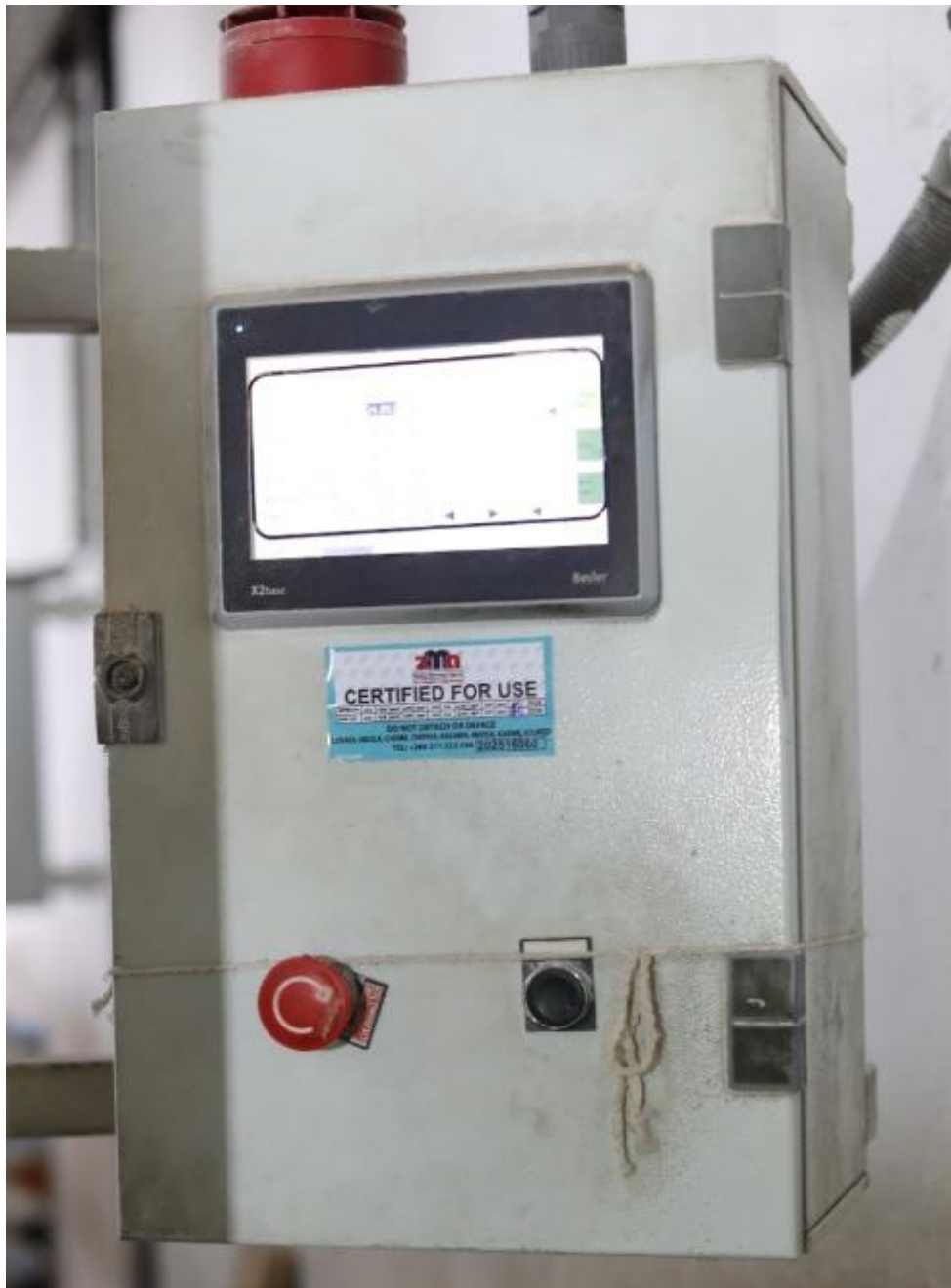
Figure 2. An example of a ZMA “Certified for Use” verification sticker on an automatic packer that dispenses a predetermined quantity of product into packages.
