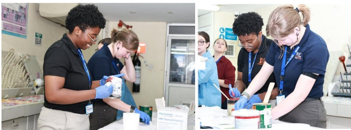
Figure 3. Lead determination in paint training at the Kenya Bureau of Standards (KEBS) laboratories.
