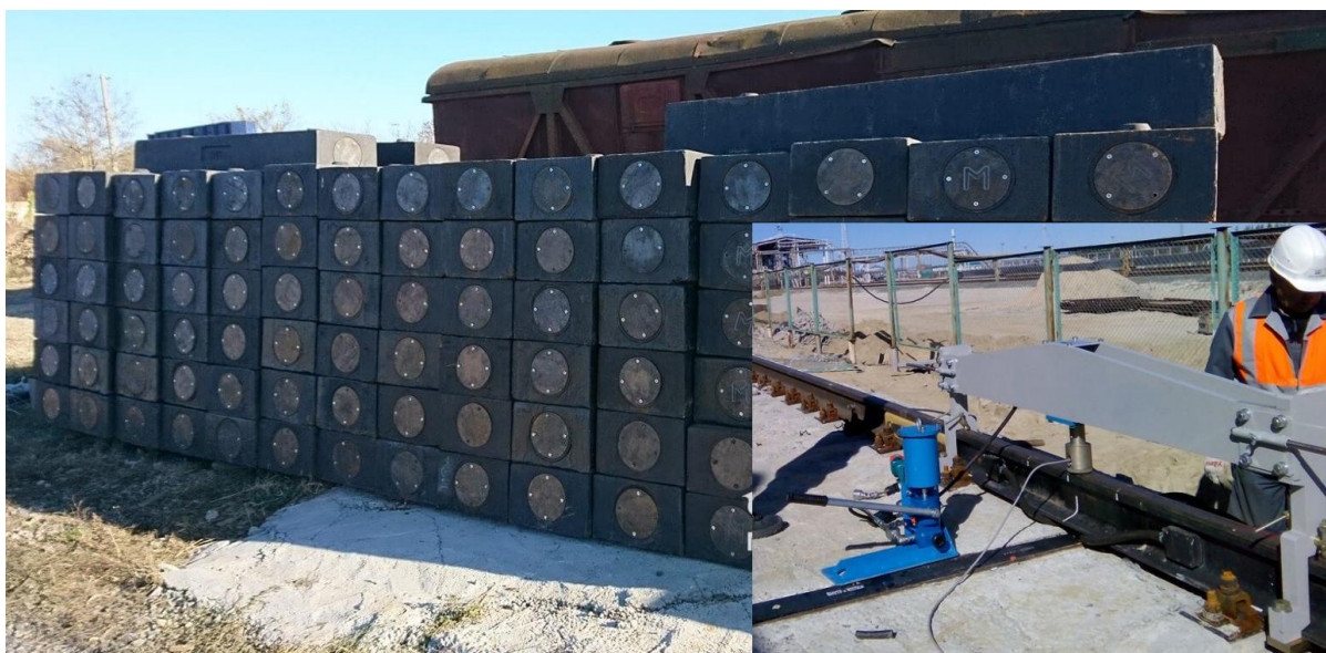
Figure 2. Verification of rail-type wagon scales: conventional and force-based methods. Reference weights used for conventional verification of wagon scales are shown on the left. The inset shows a rail load cell loaded by a transportable force-based verification standard with a nominal load of up to 12.5 t. Sequential loading of eight rail load cells enables verification of wagon scales with capacities of up to 200 t. Comparison with conventional reference-weight loading showed a difference of no more than 10 kg over the range up to 50 t.
