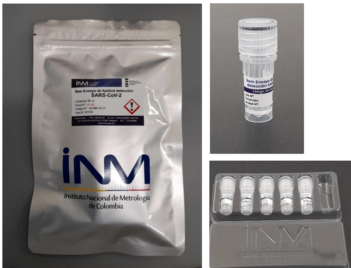
Figure 1. A proficiency test item (PTI) was developed by INM based on NIST reference material RGTM 10169 and characterized across a range of viral concentrations.
