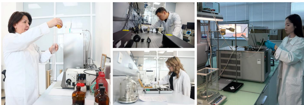
Figure 1. KazStandard metrologists performing calibrations and preparing CRMs. Left: calibration of viscosity standards. Top: calibration of a laser interferometer. Bottom: calibration of mass standards. Right: preparation of a conductivity CRM.
