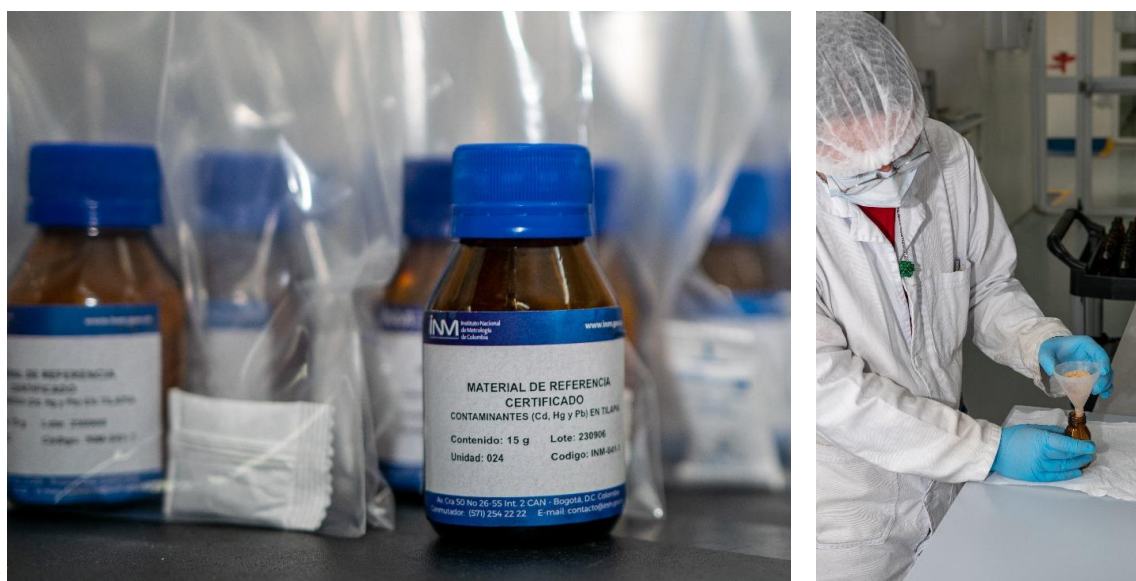
Figure 1. (a) INM Certified Reference Materials (CRMs) for Contaminants (Cd, Hg, and Pb) in Tilapia. (b) Preparation of a single CRM unit consisting of 15 g of freeze-dried, ground (to 300 mm) tilapia tissue.
