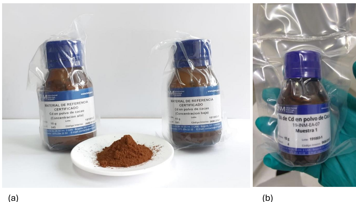
Figure 2. CRMs of cadmium in cocoa powder: (a) high and low concentrations; (b) Proficiency Test (PT) item: cadmium content in cocoa powder.
