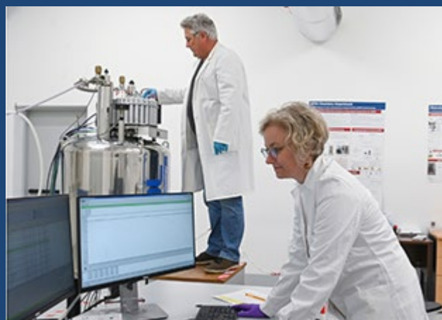
The purity of mycotoxin primary reference materials being measured with quantitative nuclear magnetic resonance (qNMR)
