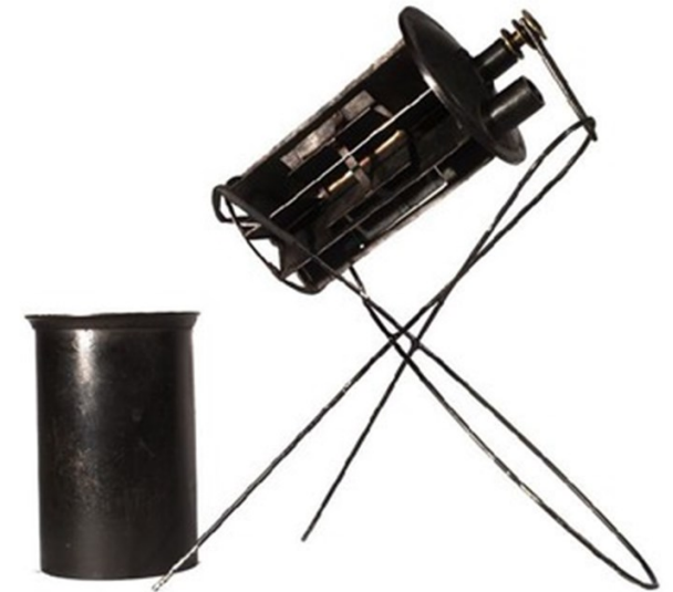
Cast Iron Paddle Wheel Apparatus; was given to Kelvin by Joule. It was used between 1847-1849 to obtain a determination of the Mechanical Equivalent of Heat. Courtesy Hunterian Museum - Glasgow GLAHM 113362
