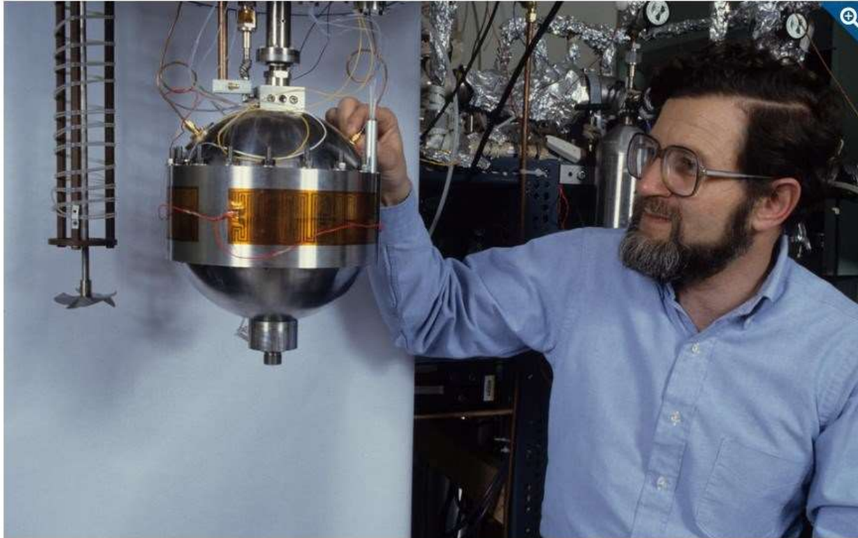
Michael Moldover and an acoustic resonator he and his colleagues developed for making some of the world's most accurate measurements of the Boltzmann constant
