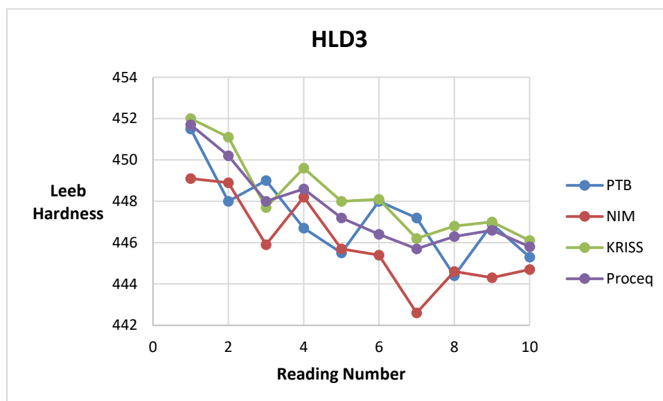
Diagram B.2: Dependence of the hardness on the number of the indentation from block HLD3
