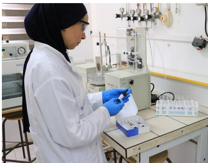
Figure 2: INRAP gravimetric unit for the preparation of certified calibration solutions
