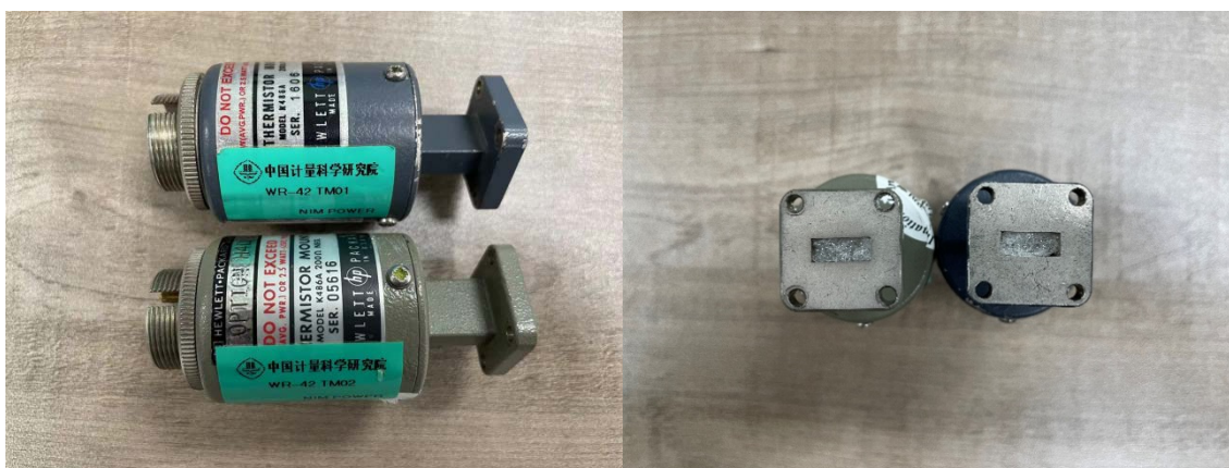
Figure 1. NIM-1 and NIM-2 travelling standards
