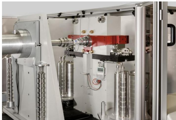
Figure 3 – PTB 1 kN·m deadweight torque standard machine
