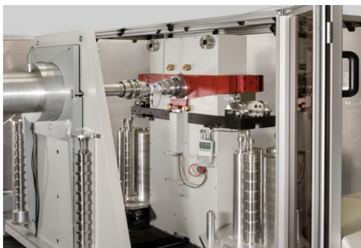
Figure 3 – PTB 1 kN·m deadweight torque standard machine
