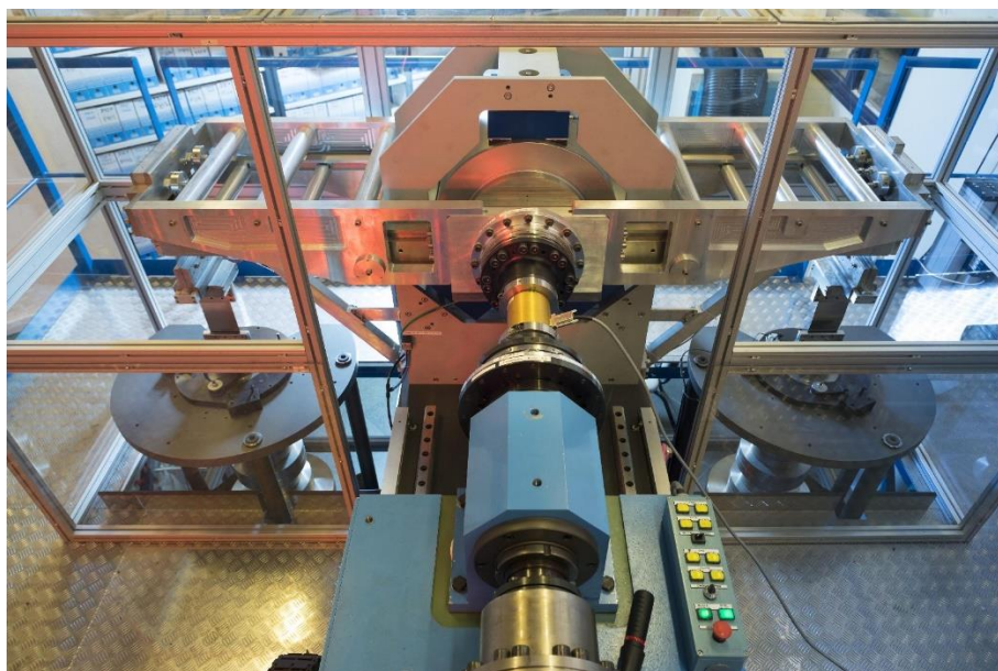
Figure 2 - LNE 500 N·m deadweight torque standard machine
