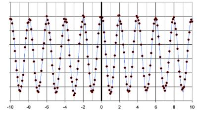
Standard launching scheme, with the MOT turned off during ballistic flight of atoms provided good Ramsey fringes (see Figure). That first version of a fountain delivered better short term stability than our current caesium beam tubes. No error budget has been made for the accuracy.
