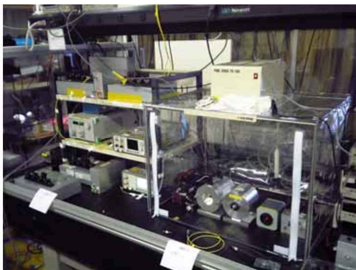
Fig. 11 Fiber power calibration system
