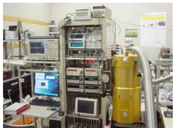
Fig. 16 Single photon detection system
