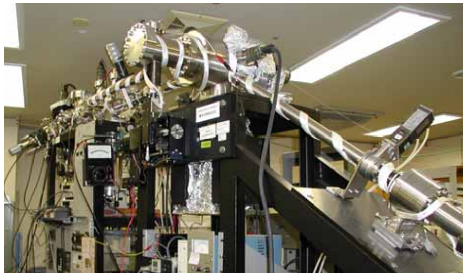
Fig. 20 VUV toroidal grating monochromator beamline for detector calibration based on ionization chamber
