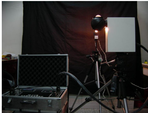
Figure 2. the standard apparatus for global solar UV spectral irradiance measurement
