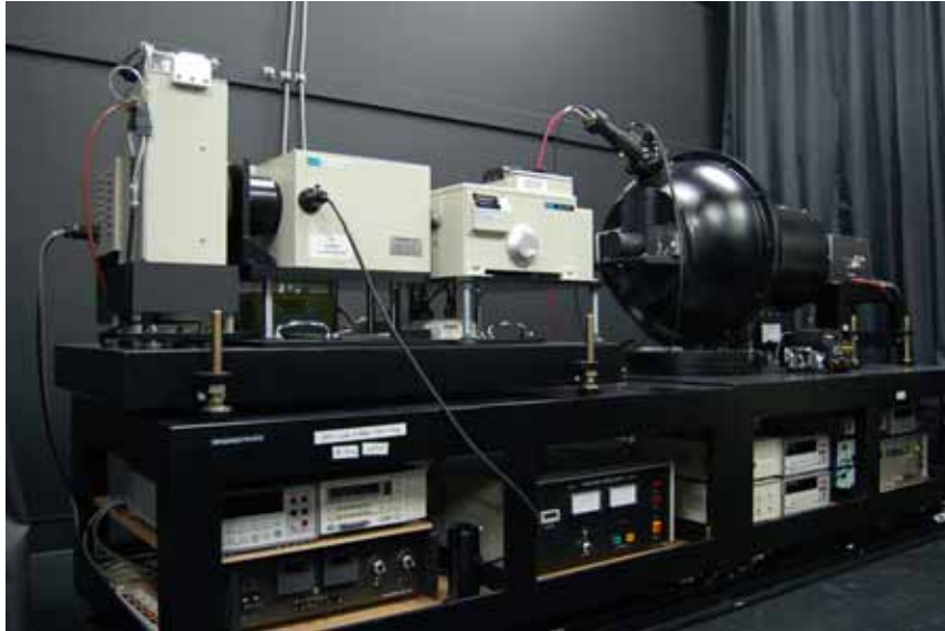
Fig. 19 NMIJ reference spectrophotometer for the calibration of spectral diffuse reflectance in the UV, VIS and NIR region
