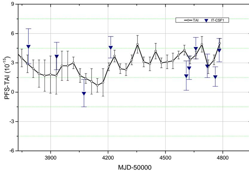
Figure 2. IT-CsF1 TAI frequency evaluations as reported in the BIPM circular T for the period 2006-2008. Triangles: IT-CsF1 frequency. Open circles + line: TAI frequency.
