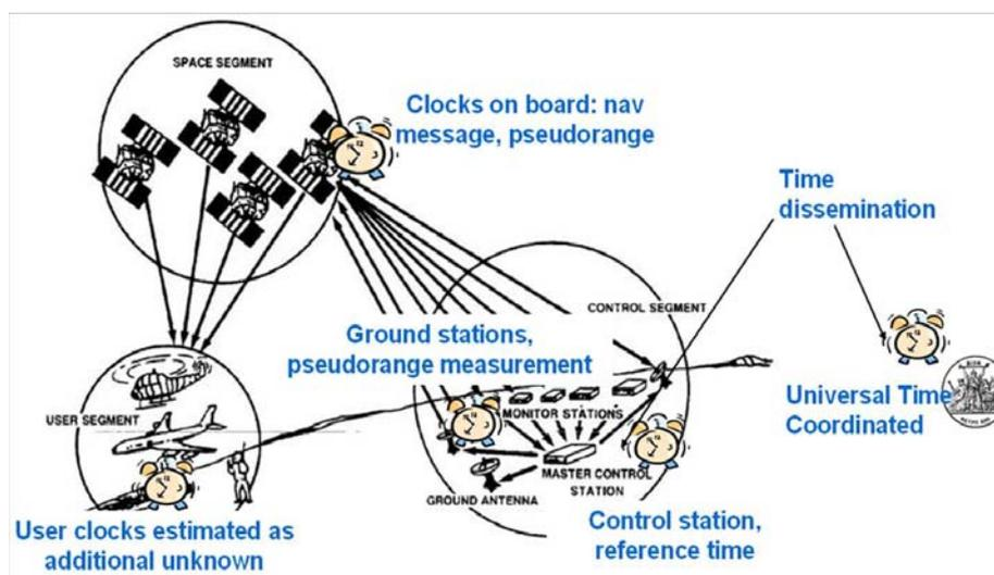
Figure 10. in the space and ground segments of a navigation system as well as in the connection to the metrological community, clocks, time scales, and time measures play a fundamental role
