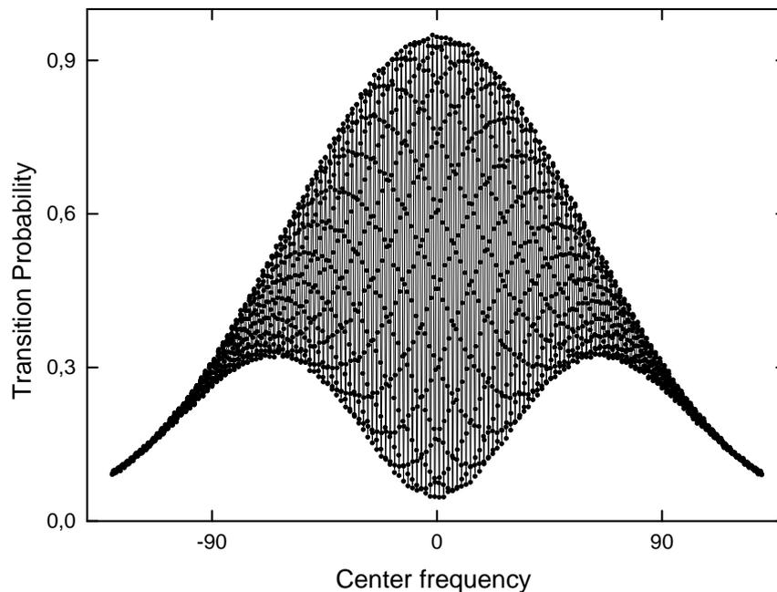
Figure 4. Ramsey fringe pattern is shown for a toss height of 1m. The corresponding Ramsey time is 550 ms yielding a linewidth of 0.9 Hz.
