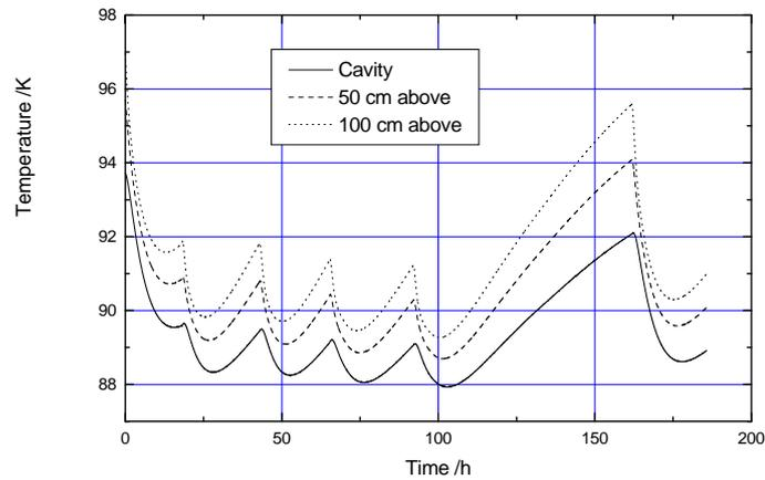
Figure 3. Time record of F2 interaction region temperatures
