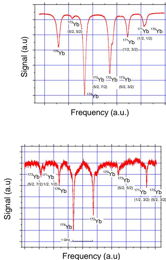
Figure 5. Yb beam spectroscopy on the  $^1\text{S}_0$ - $^1\text{P}_1$  and  $^1\text{S}_0$ - $^3\text{P}_1$  transitions
