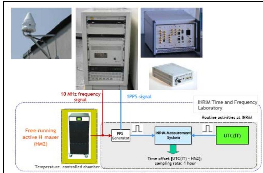
Figure 11. the prototype Galileo receiver hosted at INRIM and connected to the Italian reference time scale
