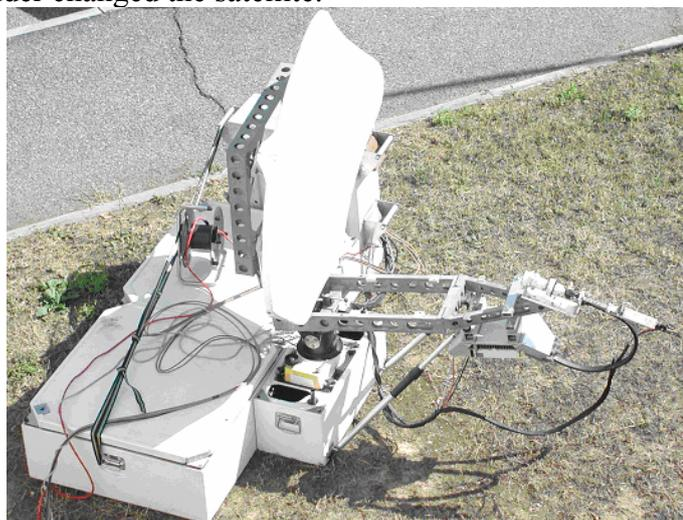
Figure 9. Transportable TWSTFT station
