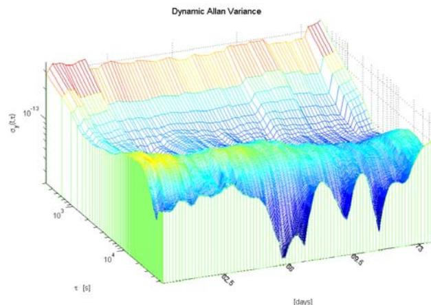
Figure 12. The Dynamic Allan Deviation extend the classical 2 dimensional analysis to a time variant system
