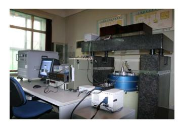
120 Hz and maximum acceleration applied is 30m/s<sup>2</sup>. The maximum peak-to-peak displacement is 40 mm for vertical exciter.
