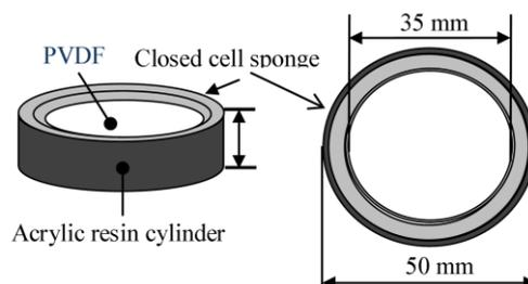
**Fig. U12** A structure of cavitation sensor with high spatial resolution.
