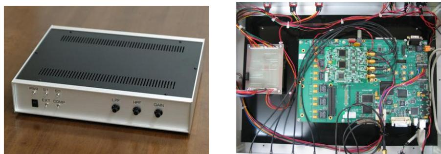
**Fig. V7** Digital demodulator for laser vibrometer standard
