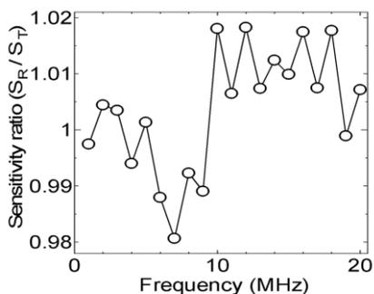
**Fig. U2** Ratio of the measured sensitivity of a membrane hydrophone by two kinds of pellicles.
