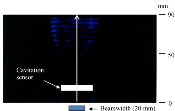
**Fig. U15** Photograph of sonochemical luminescence observed from the side of the water vessel at the frequency of 150 kHz.
