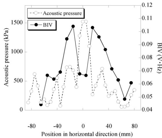
**Fig. U11** Variations of BIV and acoustic pressure along the centerline of water vessel.
