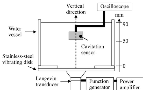
**Fig. U13** A Schematic figure of water vessel for cavitation experiments.
