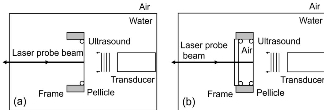
**Fig.U1 (a)** Conventional “transmission” method.
