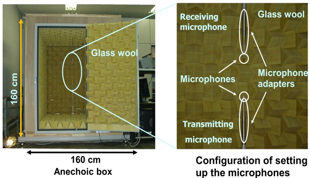
**Fig. A2** Compact anechoic chamber used for the calibration of airborne ultrasound by the reciprocity technique.
