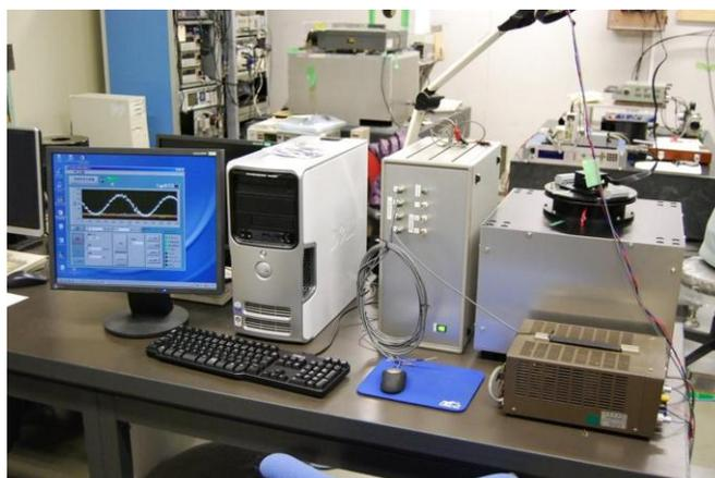
**Fig. V8** Angular velocity calibration system under development
