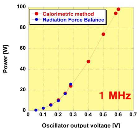
**Fig. U7** Measured ultrasonic power by radiation force balance and calorimetric method up to 100 W, 1MHz.
