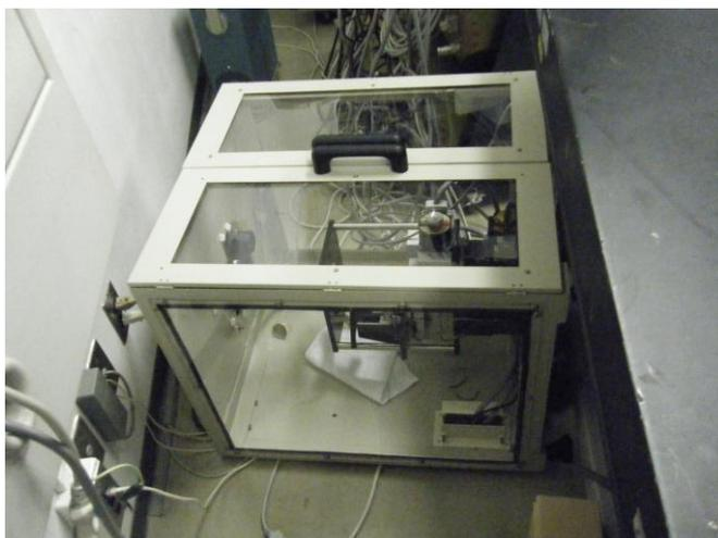
**Fig. U3** Dropped RFB system (Photographed immediately after the earthquake)
