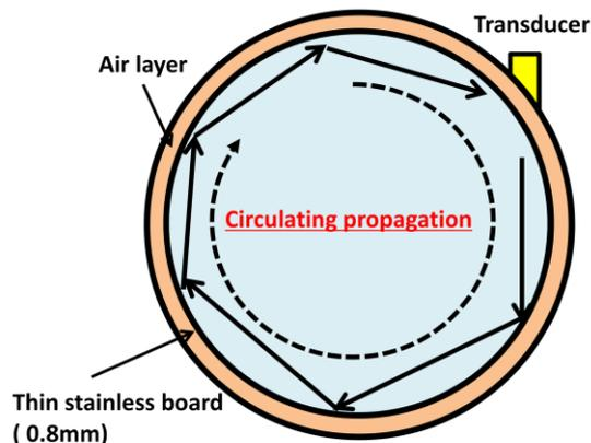
**Fig. U6** Top view of the water bath.
