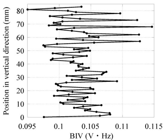
**Fig U14** Measured BIV by scanning the cavitation sensor along with the center axis of the Langevin transducer, at the frequency of 150 kHz.
