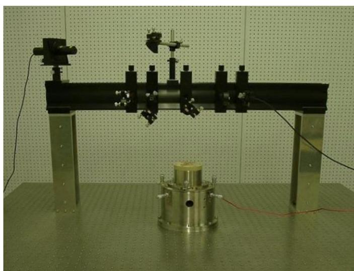
**Fig. A3** “Laser pistonphone” which composes the microphone calibration system for infrasound.
