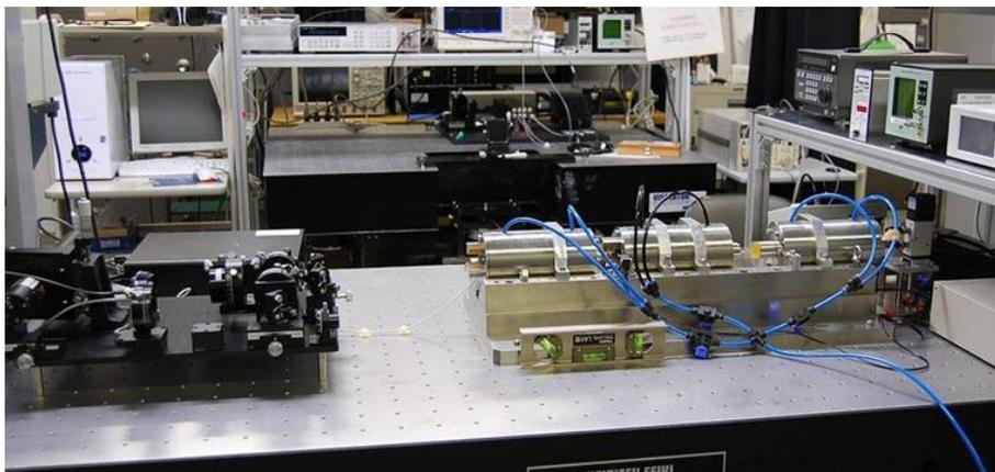
**Fig. V5** System 5: Shock acceleration calibration system
