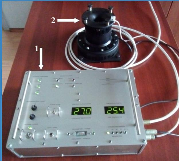
The equipment to be delivered to the ISS for realization “REPER-KALIBR” experiment with Ga-based eutectics (1<sup>st</sup> stage)
