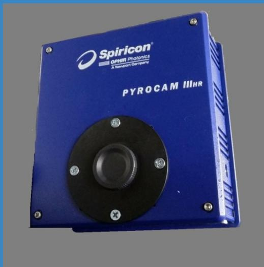
Appearance of a THz pyroelectric camera
