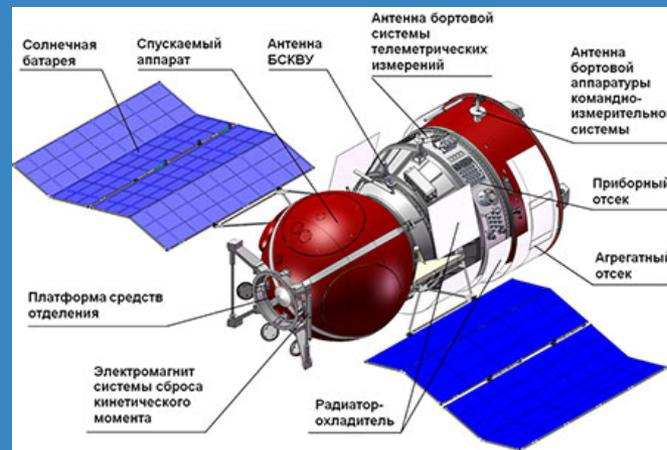
The device KALIBR designed for the flight test on board the "PHOTON-M" No.4 spacecraft
