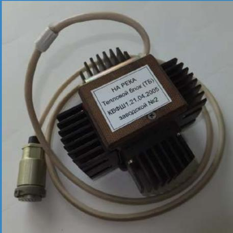
The thermal block of the equipment for realizing the flight test on board the ISS. (1-st stage)
