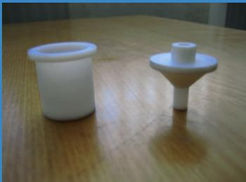
The thermal block's Teflon cell for filling with Ga and Ga-based eutectics to be studied in zero-gravity
