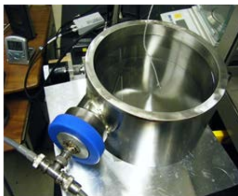
Fig. U2: A “free field“ water bath.
