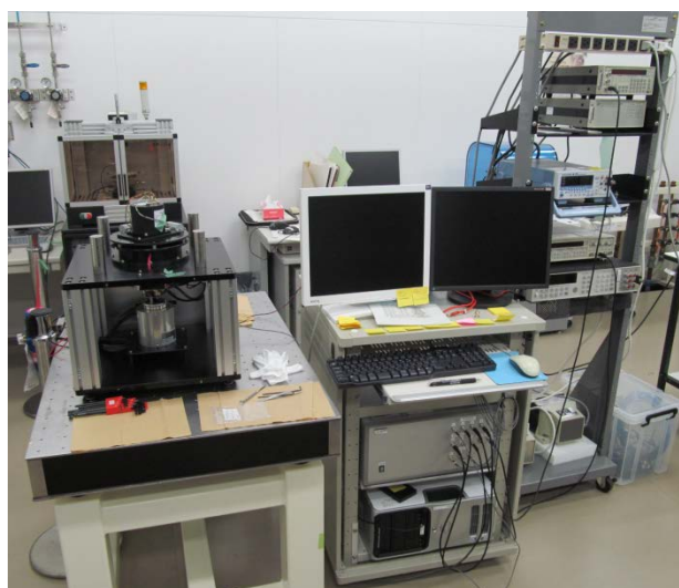
Fig. V5 System 5: Angular velocity calibration system
