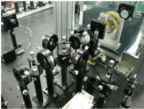
Fig. U3: A photograph of primary hydrophone sensitivity calibration system using laser interferometry.
