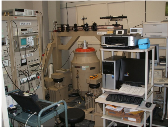
Fig. V2 System 2: Low-frequency vibration calibration system
