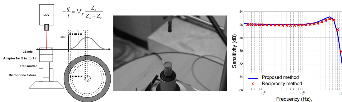
Figure 4 – System for sensitivity measurement system for LS microphone by measuring the diaphragm vibration.
