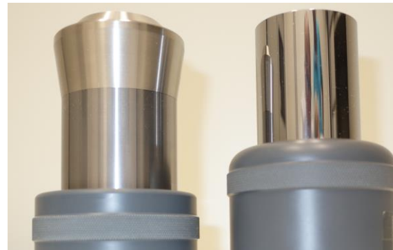
Piston cylinder assembly - 50 mm of diameter
