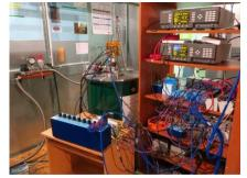
CMI also possesses CMCs for phase shift measurement in wide range of frequencies using sampling systems with multiparameter sine fitting. The setup is capable to measure up to 1 MHz. Extension to 100 MHz is planned in 2019 – 2020.
