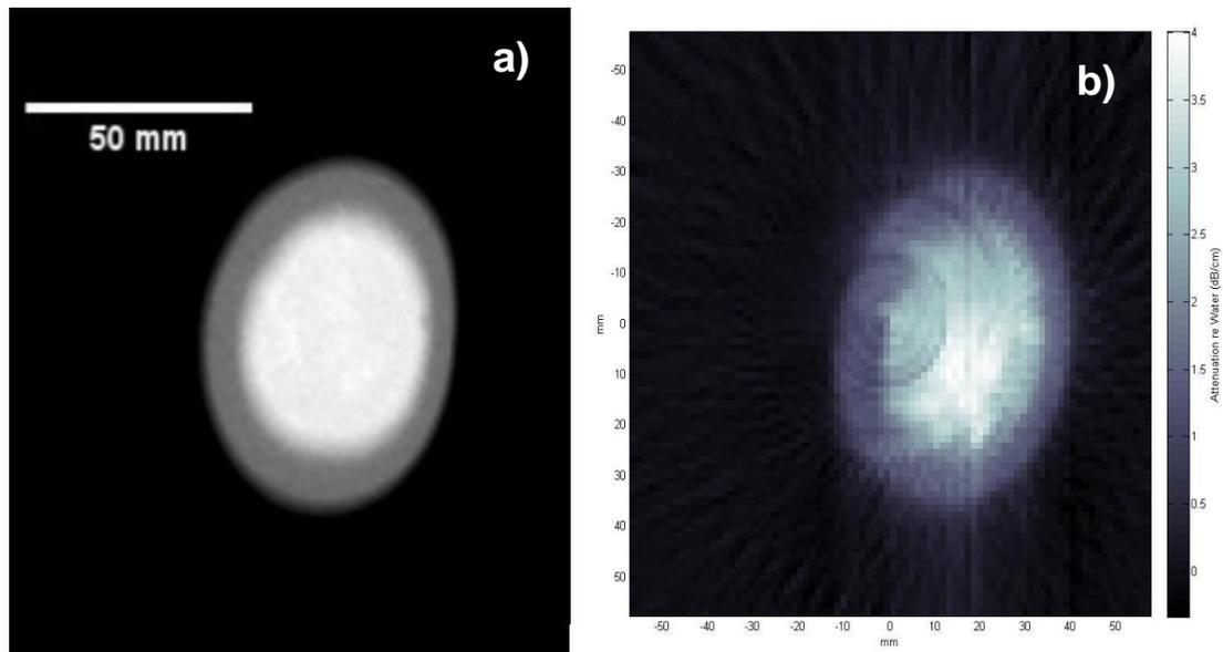
Fig 7. A comparison of two imaging modalities on a CIRS Model 043 breast phantom in the frontal plane at  $z = 17\text{mm}$  by: a) XCT and b) piUCT scans.
