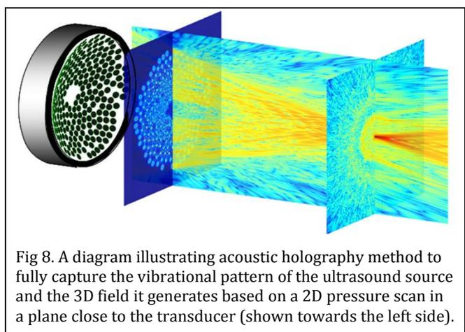
Fig 8. A diagram illustrating acoustic holography method to fully capture the vibrational pattern of the ultrasound source and the 3D field it generates based on a 2D pressure scan in a plane close to the transducer (shown towards the left side).
