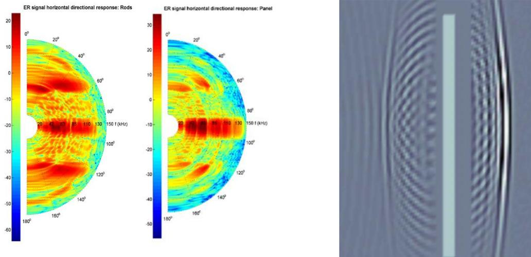
Fig 3. Echo Reduction polar frequency response for two test objects with periodic structure (left) with amplitude shown as colour map and frequency shown along the radius; On the right is shown an experimental nearfield scan of one of the test objects showing the transmitted and reflected waves, including the scattered waves generated by a diffraction grating effect of the periodic structure.
