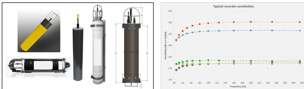
Fig.2 Images of typical marine autonomous acoustic recorders (left) and the results of calibration of such units in the frequency range 20 Hz to 315 Hz (left).
