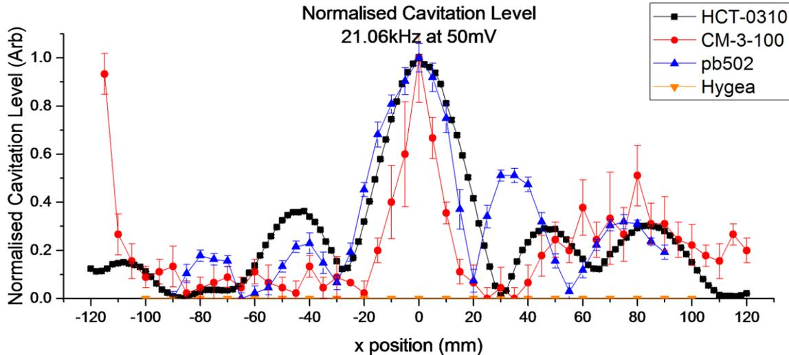
Fig 10. A comparison of normalised cavitation level as measured by the commercially-available cavitation meters at 50 mV drive. Plotted error bars are  $\pm 1$  standard deviation. Note: the HCT-0310 error bars are too small to be visible on this plot.
