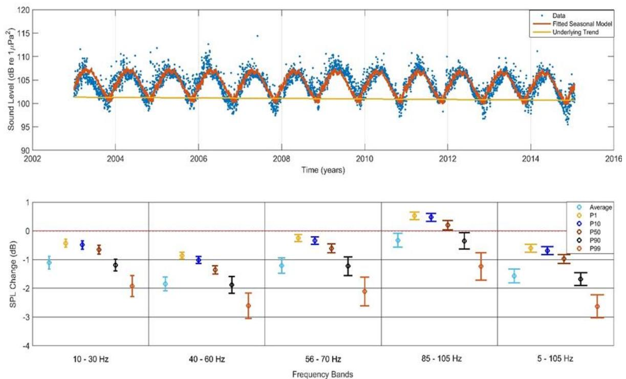
Fig. 1 Measured time series (upper) and estimation of trends in the mean and 5 different percentiles in ocean ambient noise and quantification of the estimates' uncertainties through application of regression with bootstrap resampling of the residuals (lower).
