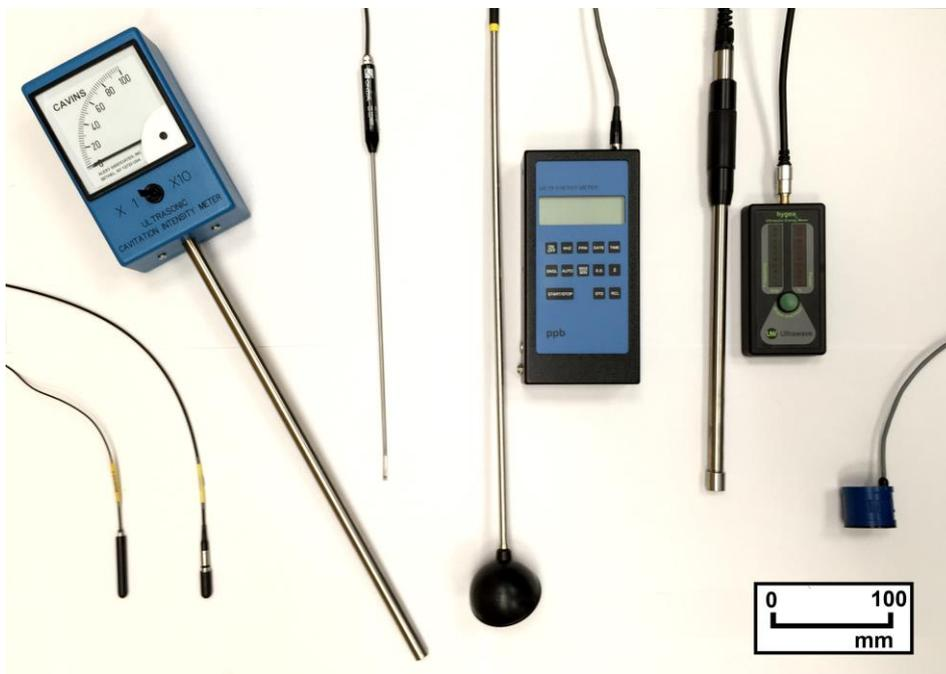
Fig 9. Photograph of the hydrophones and commercial cavitation meters used in this study. From left to right: TC4038, TC4013, CM-3-100, HCT-0310, pb502, Hygea Ultrasonic Activity Meter and CaviSensor™.
