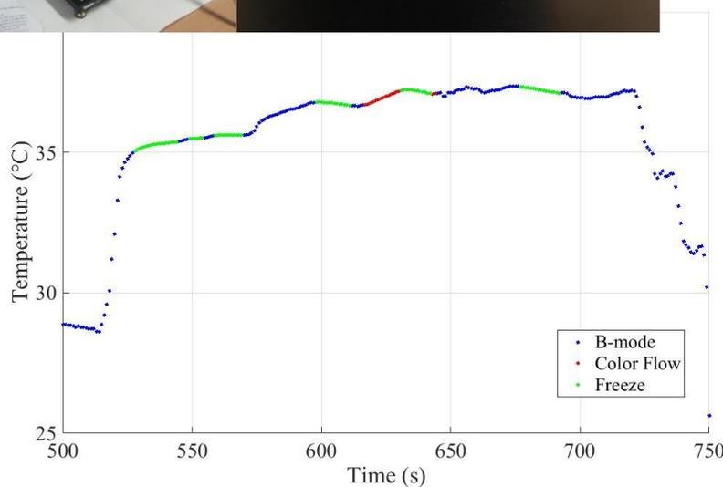
Fig 5. Example of a temperature curve at the surface of the probe during an *in-vivo* scan. Active modes obtained from the images are highlighted
