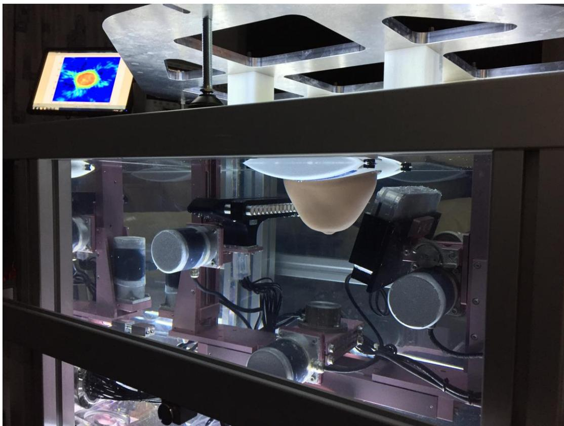
Fig 6. Image of the CIRS breast phantom deployed with the piUCT water-tank, between the angled large single element area sensor (right-hand side) and the linear transducer array (left-hand side).
