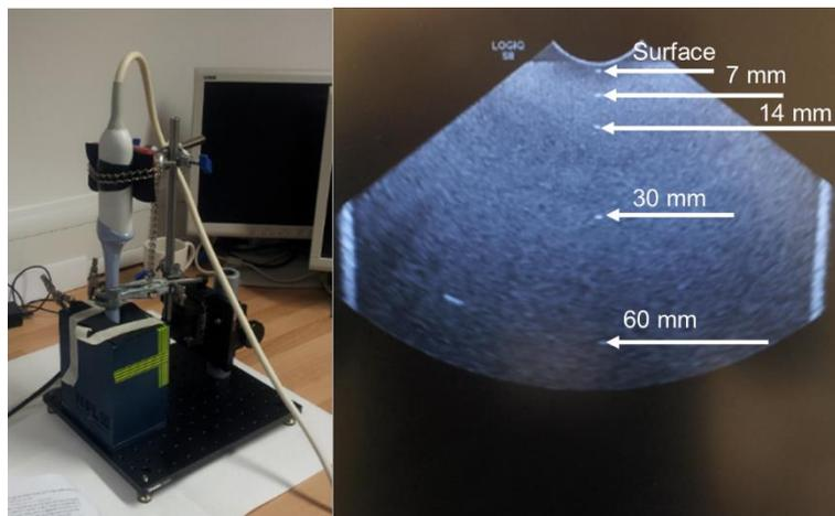
Fig 4. The phantom developed for the assessment of commercial probes (left) and an ultrasound image of the Tissue Mimicking Material block with the 5 fine wire thermocouples embedded at the indicated depths within the block.
