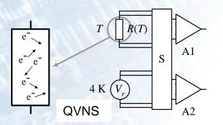
(Quantum-accurate pseudorandom Voltage-Noise Source traceable to voltage standard)
