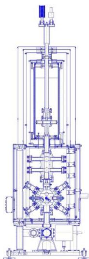
low 1  $\mu$ K. The laser beams locates in two mutually orthogonal planes with beams angle relative to vertical axe about 1 radian. The main aim of such beams configuration is a desire to get more spherical shape of Cs cold atom cloud.
