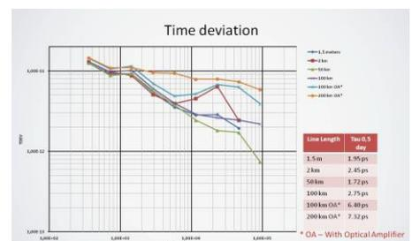
The experiment demonstrated ability to get time resolution  $\sim 10^{-12}$  s for sample time about 1 day.
