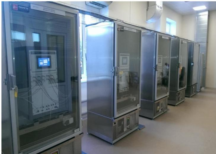
company [4]. That include ensemble of high quality H-masers (each in temperature/humidity control housing), distributing T&F amplifiers and time and frequency inter comparison system. Preliminary performance tests based yielded following results:
