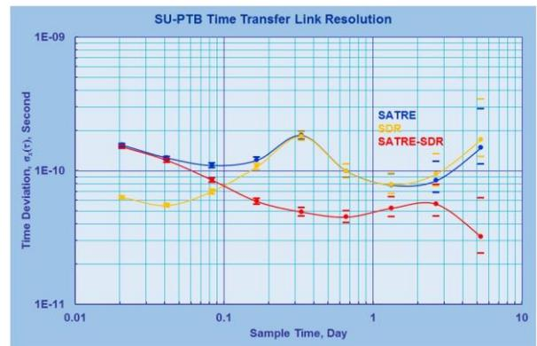
noise component for SDR. Diurnal component still presents both in SATRE and SDR data. Red curve at the right figure demonstrates random residuals in SATRE-SDR links. If one will succeed in suppression diurnal component SDR link performance will be considerably better than  $1 \times 10^{-10}$  s for any sample time starting from session repetition up to a few days.
