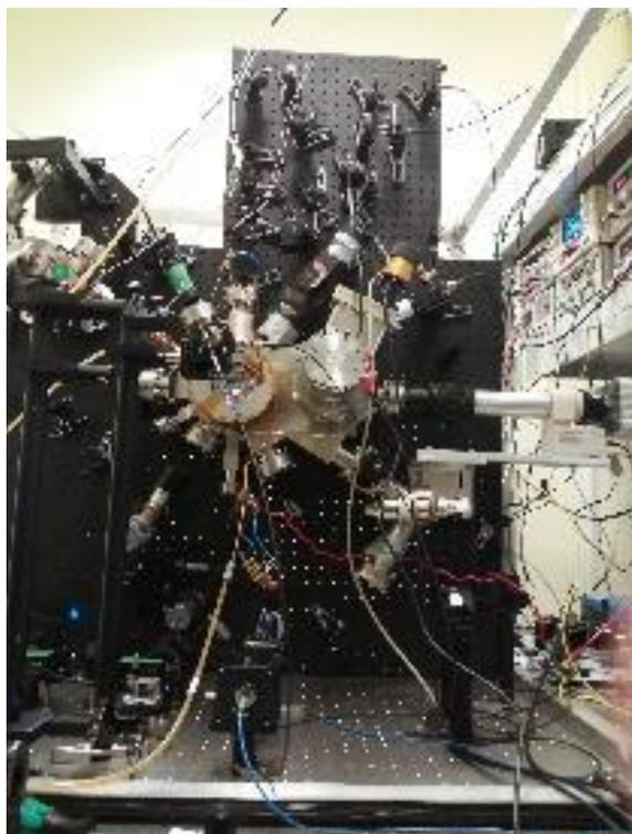
The vertical wall at attached picture hosts optical spectroscopy chamber with optical lattice system and clock transition laser detection system.
