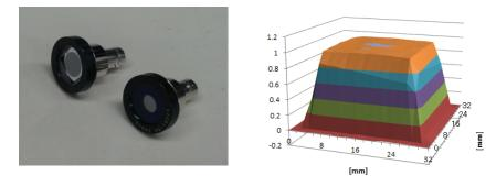
Radiant flux standard (W) in UV region was realized by using a blackbody radiator and a monochromator. A deuterium lamp is used for transfer standard and that radiant flux in 20 nm wavelength width can be calibrated from 180 nm to 320 nm.
