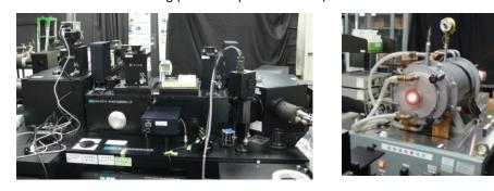
BRDF scale for white diffuser plate in a limited geometry was established. The angles of incident radiation and reflected radiation are 0 degree and 45 degree respectively. The BRDF calibration is available form 360 nm to 830 nm.
