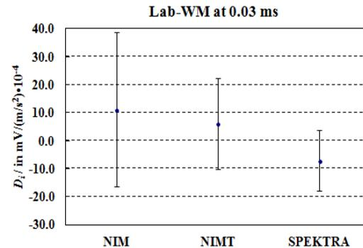
Degree of equivalence for voltage sensitivities under dipole shock excitation at 1000 m/s<sup>2</sup>, 0.20 ms and 0.03 ms
