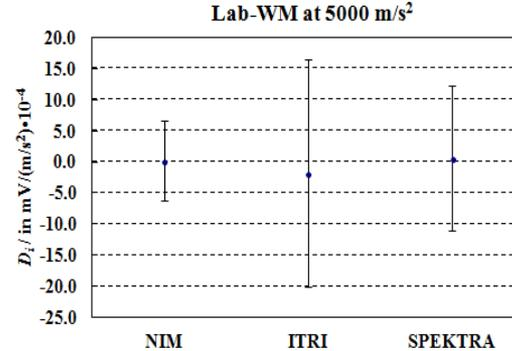
Degree of equivalence for voltage sensitivities under monopole shock excitation at 1000 m/s<sup>2</sup>, 2.0 ms and 5000 m/s<sup>2</sup>, 0.8 ms
