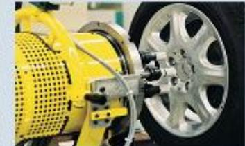
Sinusoidal torque under rotating and non-rotating conditions
