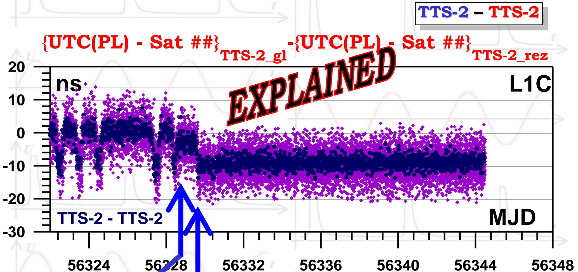
1. the change of localization of GPS receiver and antenna cable (further away from the monitor)
