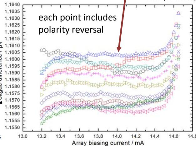
voltage of JVS remains quantized on the Shapiro step in the complex electrical environment of the watt balance
