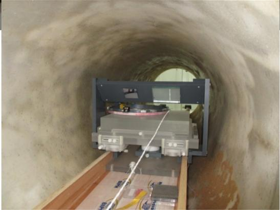
Watt balance coil inside the solenoid
