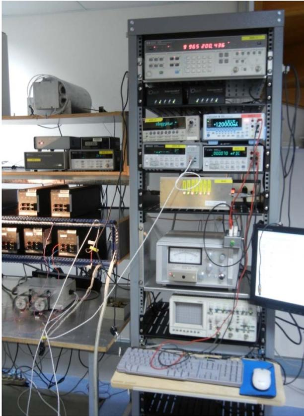
Automated BIPM Zener measurement setup based on a PTB – programmable Josephson Voltage Standard
