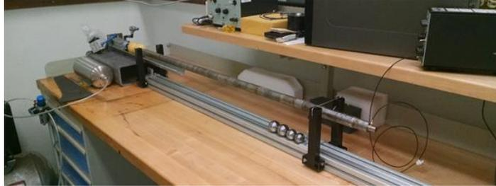
Figure 1.5. Hopkinson bar for calibrations by high-intensity shocks.
