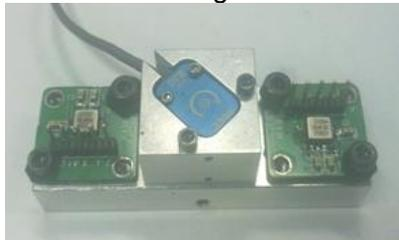
Figure 1.6. Comparing two rectilinear MEMS accelerometers and one angular rate sensor.
