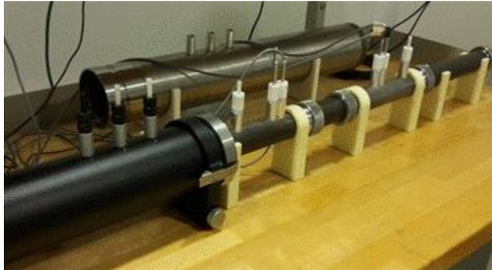
Figure 2.6 Impedance tube built at CENAM.
