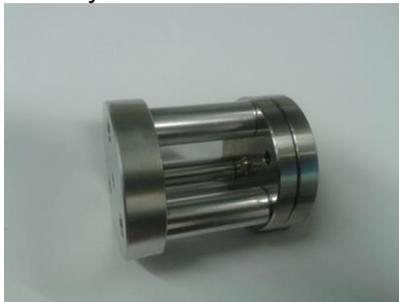
Figure 1.7. Mounting fixture to calibrate accelerometers by comparison (10 Hz – 10 kHz).
