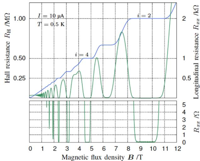
Fig. 3 Picture and Hall and longitudinal resistance curve of 1 M $\Omega$  array device.
