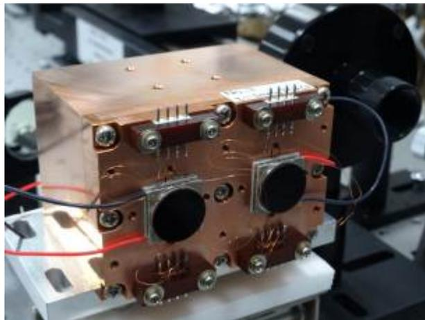
Fig. 9 Prototype of Twin type THz Calorimeter
