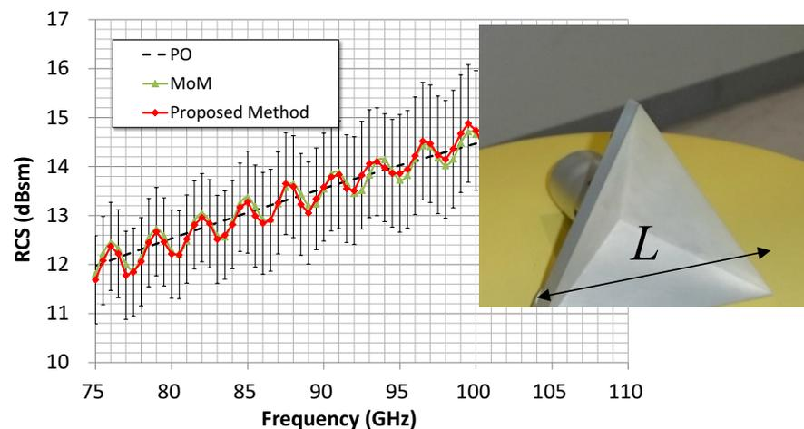
Fig. 7 RCS calibration results in W-band and an example of a trihedral corner reflector
