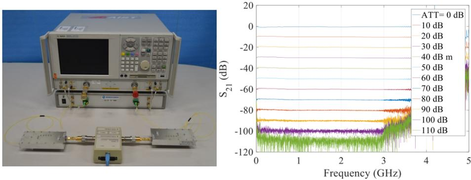
Fig. 8 Bi-directional RoF transceiver attached to a Vector network analyzer
