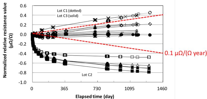
Fig. 2 Resistance histories (drifts) of 1 $\Omega$  resistors.
