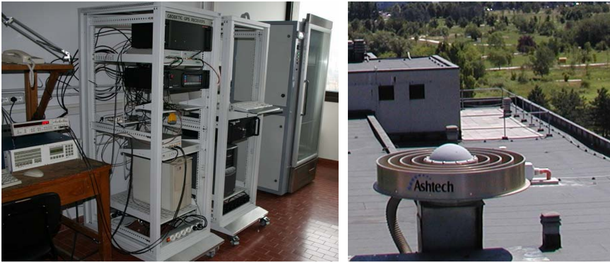
Figure 8 – INRIM GPS Laboratory with climate chamber and outdoor receiving antenna
