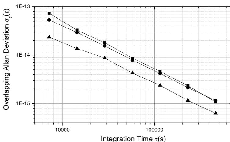
**Figure 4.** Allan deviations of double frequency differences in remote masers frequency comparison (see text), for the masers pairs NPL-INRIM (Squares), SYRTE-INRIM (Circles), NPL-SYRTE (Triangles), using TWSTFT and GPS-CP techniques.
