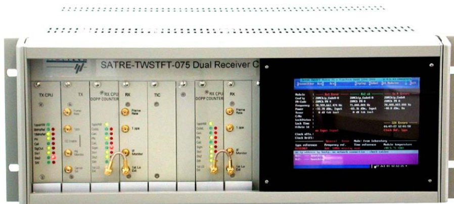
Figure 9 – Front view of the SATRE Modem used at INRIM
