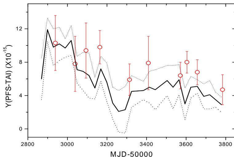
**Figure 2.** IEN-CsF1 TAI frequency evaluations since 2003 (MJD 52800 = 10/06/2003) reported on BIPM circulars T. Circles: IEN-CsF1 evaluations. Solid line: TAI frequency. Dot lines: upper and lower TAI uncertainty ( $1\sigma$ ).
