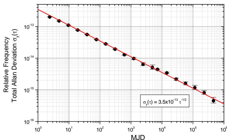
**Figure 3.** IEN-CsF1 vs IEN-HM2 relative frequency instability
