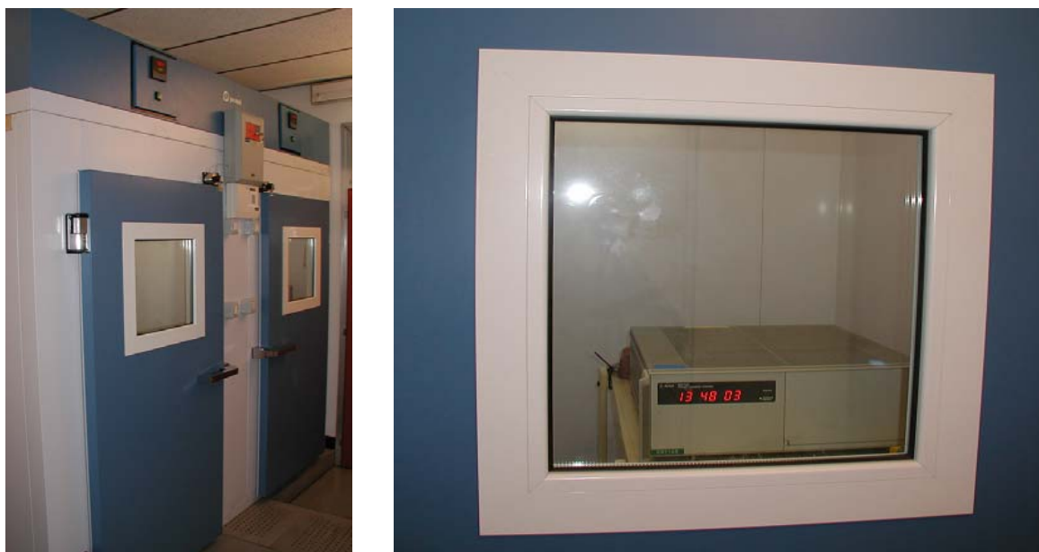
Figure 6 – Temperature controlled room for INRIM master clock up to June 2006
