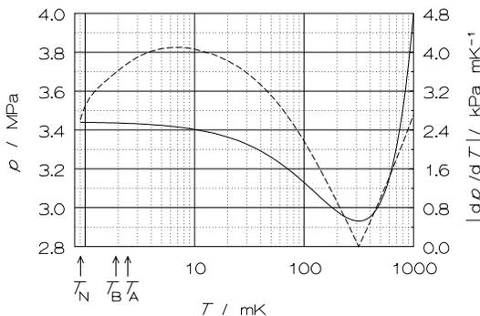
Fig. 1. The  $^3\text{He}$  melting pressure,  $p$ , (full line) and the absolute value of the derivative  $dp/dT$  (dashed line) versus temperature.  $T_N$ ,  $T_B$  and  $T_A$  indicate the temperatures of three phase transitions in solid or liquid  $^3\text{He}$ .
