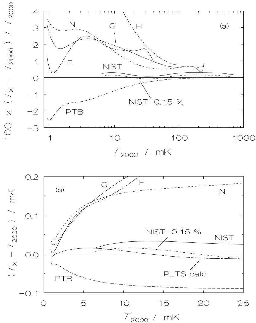
Fig. 2. a) Relative differences between laboratory scales and the PLTS-2000 as a function of temperature. H: Halperin<sup>2</sup>, G: Greywall<sup>3</sup>, F: Fukuyama et al.<sup>20</sup>, NIST: NIST-98<sup>4</sup> before and after reduction by 0.15% of  $T$  (see text), N: UF-95<sup>5</sup>, PTB: PTB-96<sup>6</sup>, all scales being defined by melting pressure equations. b) Absolute differences below 25 mK, including a comparison with a thermodynamic calculation, 'PLTS calc' (see text).
